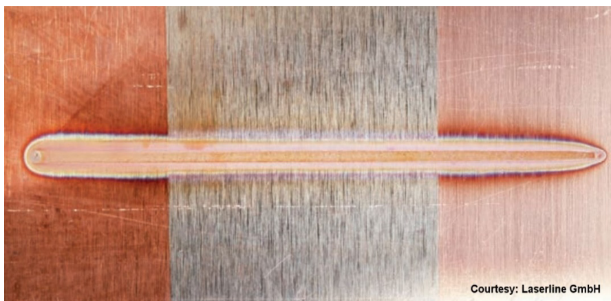
Fig. 5. Smooth and extremely stable weld of copper sheet prepared with three different surface conditions (etched, oxidized, polished)
