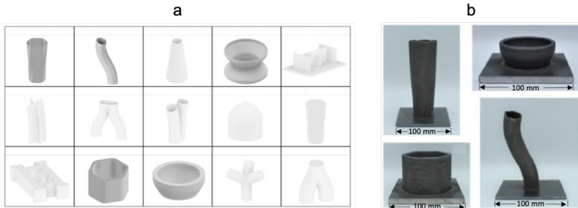
Fig. 2. (a) Categorized forms in the analysis of robotic powder LMD, (b) LMD printed exemplars of some categorized forms.
