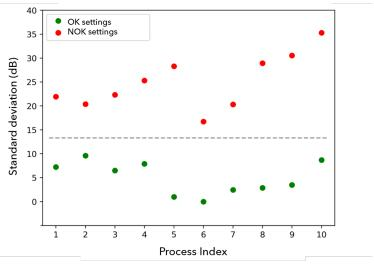
Fig. 2. Diagram of the standard deviations of the acoustic energies emitted by welding processes with good settings (marked in green) and with faulty settings (marked in red)
