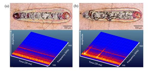
Fig. 1. (a) Picture of a good weld seam with the spectrogram of its acoustic emissions; (b) Picture and spectrogram of a faulty weld seam
