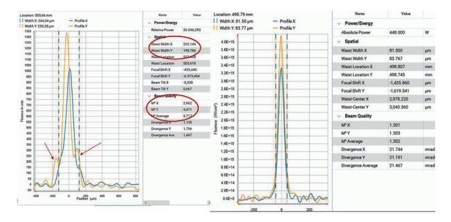
Fig. 4. Measurements on an SLM system at the Fraunhofer IAPT: On the left the laser system with quality problems, on the right the laser system with perfect results (©Fraunhofer IAPT)
