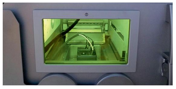
Fig. 2. Production chamber of an SLM system at the Fraunhofer IAPT (©Fraunhofer IAPT)
