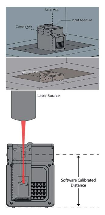
Fig. 3. Measuring principle and application of non-contact beam measurement.
