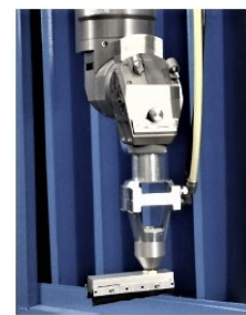
Gas shoe shield arrangement mainly used for welding titanium based alloy
