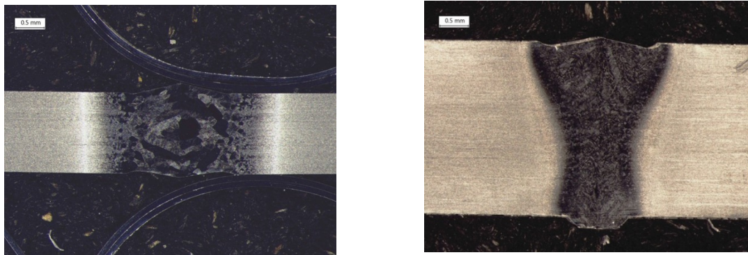
1.4mm thick Ti-6Al-4V alloy; welding speed 2.3m/min
