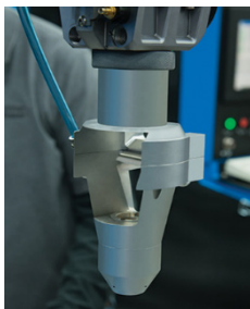
Coaxially gas shield arrangement mainly used
