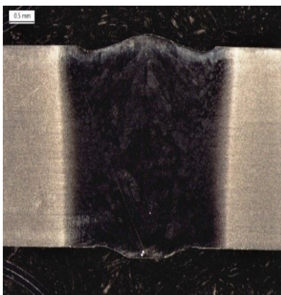
Autogenous weld; undercut and few bores
