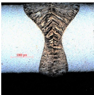
2.3mm thick Inconel 718; welding speed 2m/min
