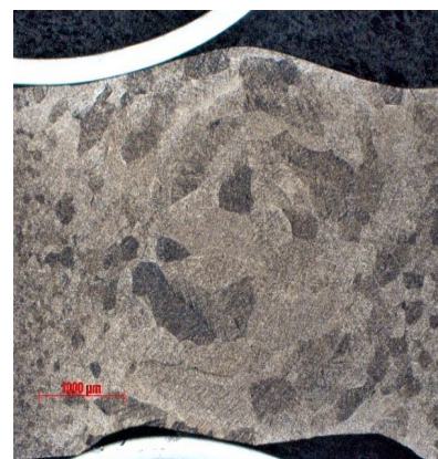
Weld made with filler material; no pores and undercut
