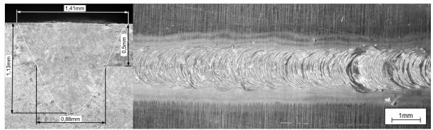
Fig. 6. ARM laser, v = 5 m/min, cross section and weld surface.
