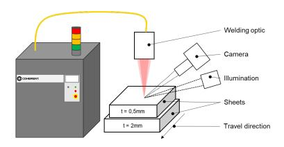
Fig. 3. Schematic experimental setup.
