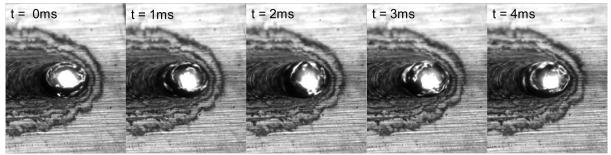
Fig. 7. ARM laser, v = 3 m/min, process observation using high speed camera.
