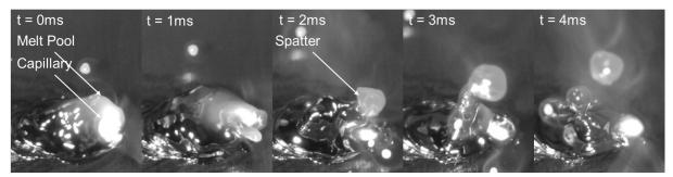
Fig. 4. Reference process, v = 6 m/min, process observation using high speed camera.
