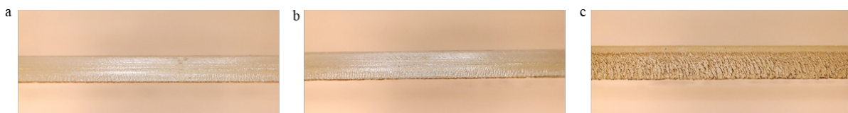
Fig. 7. (a) standard grade PC (b) UV-stabilized PC (c) flame-retardant PC.
