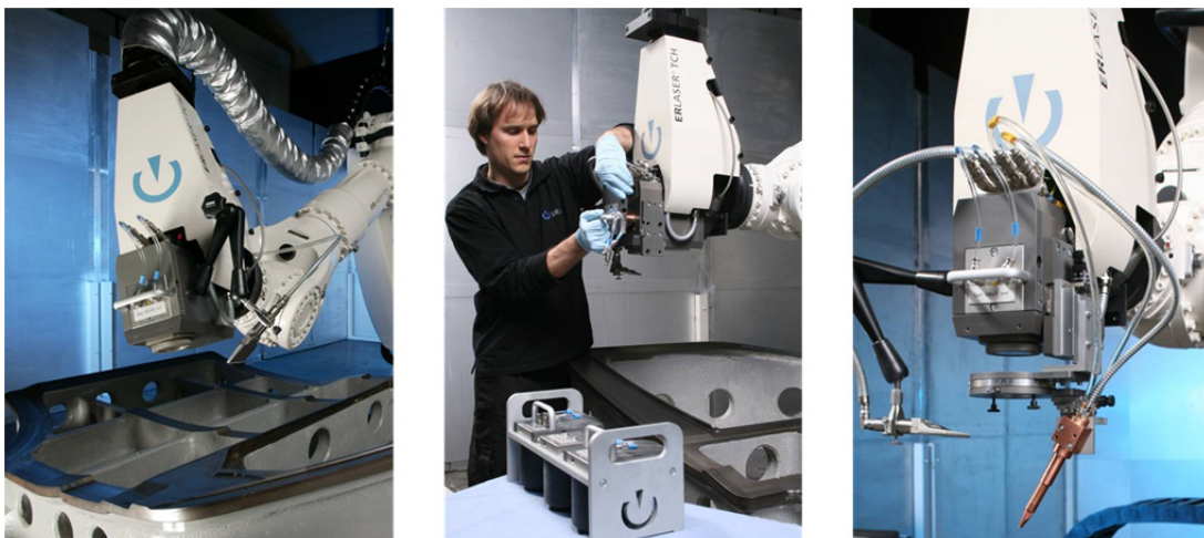
Fig. 2-4 show the conversion from laser hardening set up to laser cladding set up. An exchange of the focusing mirror and an installation of the powder feeding nozzle is necessary.
