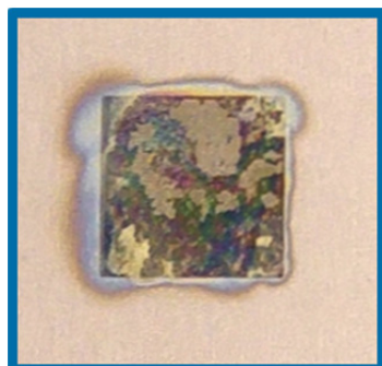
Fig. 3. Oxidation effects in nanosecond lasermarking after steam sterilization
