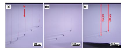
Fig. 8. Cross sections of modification lines in silicon at various depths with pulse energy (measured before the objective lens) of (a)  $2.5 \mu$ J, (b)  $2 \mu$ J, and (c)  $1.5 \mu$ J. Regions in black color and aligned vertically are laser-induced modification. Narrow vertical lines in red color are depth measurements.
