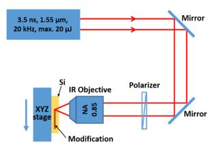
Fig. 7. Experimental setup.
