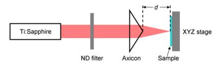
Fig. 1. Experimental setup.
