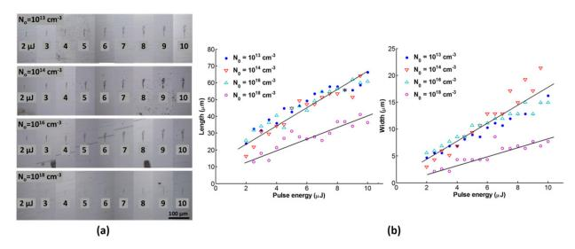
Fig. 10. (a) Laser-induced modification in silicon wafers with various level of doping (free carrier density,  $N_{o}$ , indicated in the top left of each subfigure). Pulse energy is indicated on the bottom of each modification. (b) Measured length and width of modified region at various doping levels. Solid lines are a guide to the eye.
