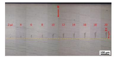
Fig. 9. Laser-induced modification at the same depth (400  $\mu$ m) and with increasing pulse energy. The horizontal dashed line marks the focusing depth. Laser polarization is random. Width (W) and length (L) of modified region are measured as depicted. Numbers above modified regions represent pulse energy in  $\mu$ J.
