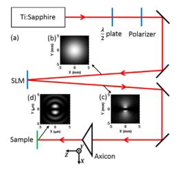
Fig. 4. (a) Experimental setup. Insets are calculated beam shapes (b) in front of SLM, (c) 1.2 m after SLM, and (d) 9 mm after axicon, respectively, for the 1+(1) superposition.
