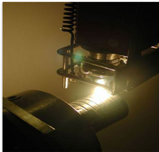
Fig. 3. Diode laser welding of a catalytic converter. (courtesy of Ecocat).
