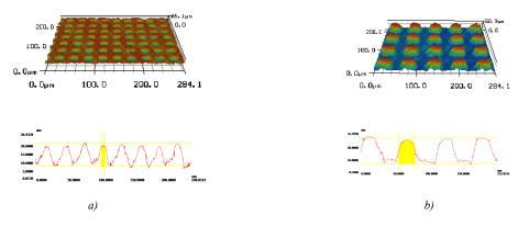
Fig. 1. (a) master structure (stainless steel) generated by laser ablation (b) replication by injection molding (PLGA)
