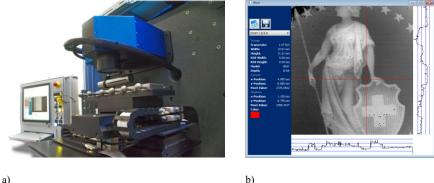
Fig. 5. (a) industrial solution of combined laser galvanometer scanner and FD-OCT (b) 3D profile measuring of a coin by FD-OCT measuring.
